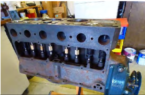
Of special interest are the "custom" made valve stem "extenders" for the SB Chevy valves that fit, but are about 1/2" short.
